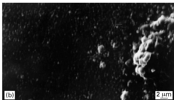
Figure 7 The scanning electron micrographs for CIS formed by selenization of (a) Cu–In, (b) Cu/In and (c) In/Cu precursors, (Magnifications, 1500x.)
